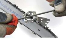
FILING THE CUTTING TEETH File using light and even pressure, with gentle pushing strokes. parallel to the gauge. Try to get the same length of all cutters.
